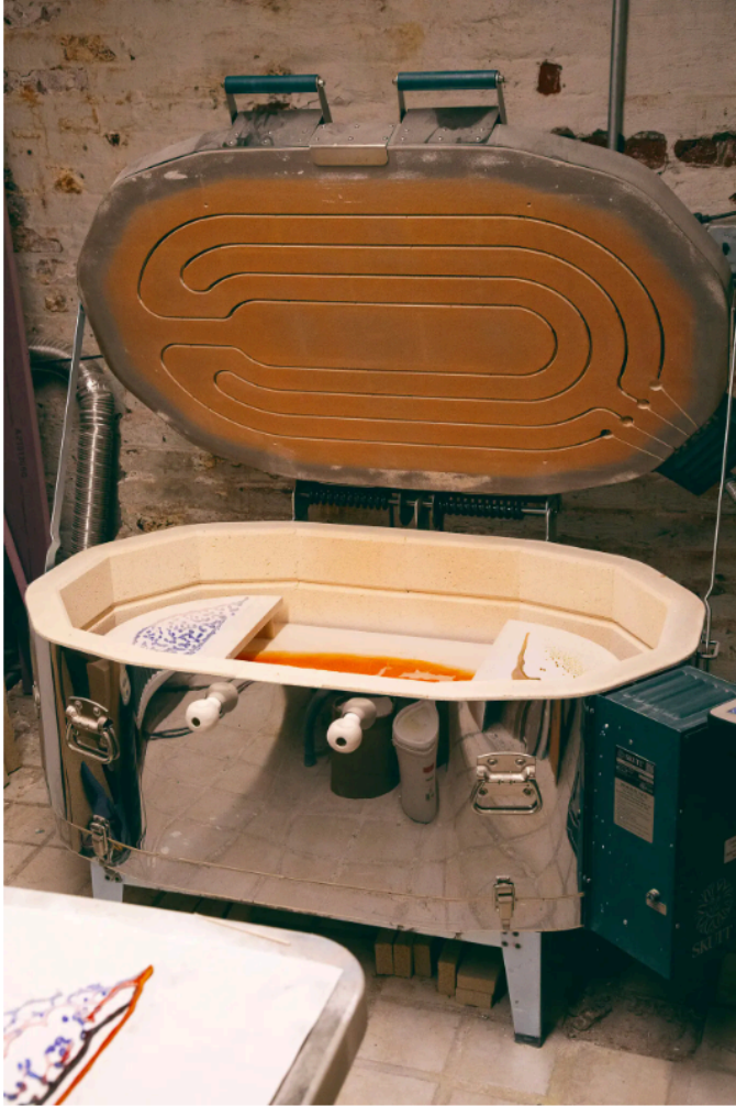
Auerbach's glass kiln, in the building's basement. Inside are just-baked examples of the frit lace they've been making using granulated glass. Melody Melamed
